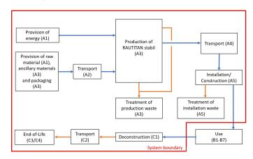
The following is a detailed list of the life cycle stages and process modules taken into account for the production of the pipe:
